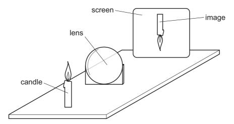
Various sharp images are produced on the screen by moving the lens and the screen backwards and forwards.
